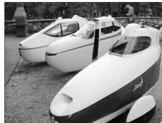
Different velomobiles present at meeting in Oktober 2000 in Germany. From front to rear: Leitra, Aeolos and Cab-bike. In contrast to the other vehicles, Aeolos (a development of the author) is a two-wheeler. Further informations can be found at http://www.velomobile.de
