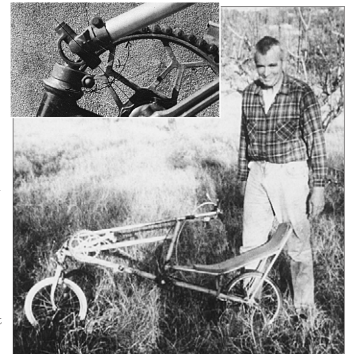
Figure 2. The first Velocar replica. Figure 3. (Inset). The original Velocar (patented) steering joint
