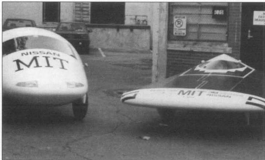
Figure 2: Among the vehicles raced by the author are the championship winning cars: the Manta solar car (right) and the 2-seat EV Aztec. The Aztec was based on the famous Morelli shape which has been used by HPV racers. (Photo: I. Gregoratto)
