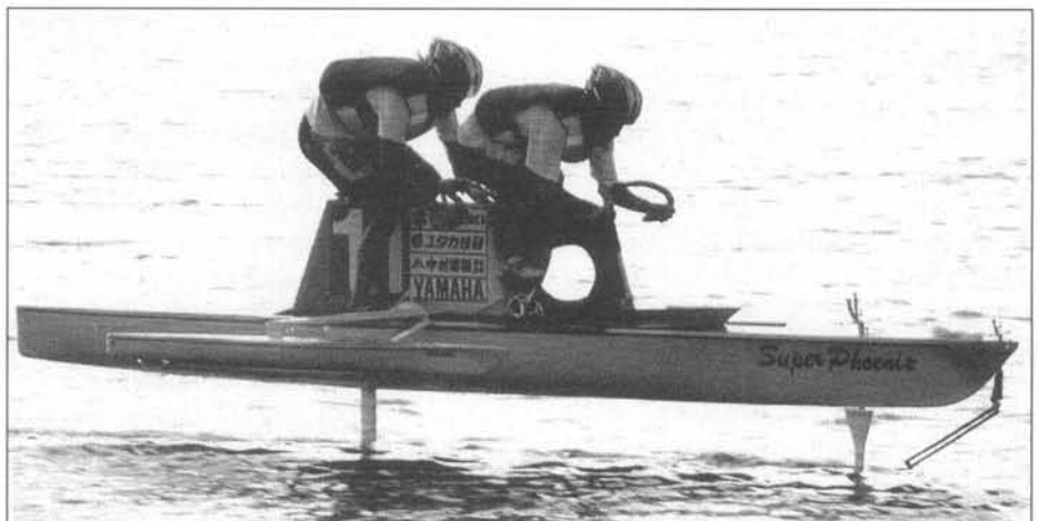
Tandem human-powered hydrofoil from a Yamaha team, competing in the 1997 human-powered boat race on Lake Hamana, Japan. Photo, courtesy Toshio Kataoka.
