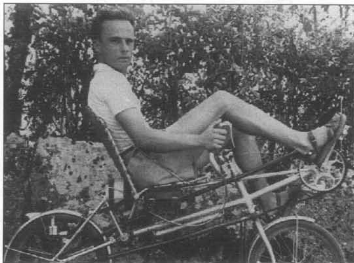
Lucien Battarel on Sliperette 1 in 1950. Both wheels had suspension; the chain ran in tubes
