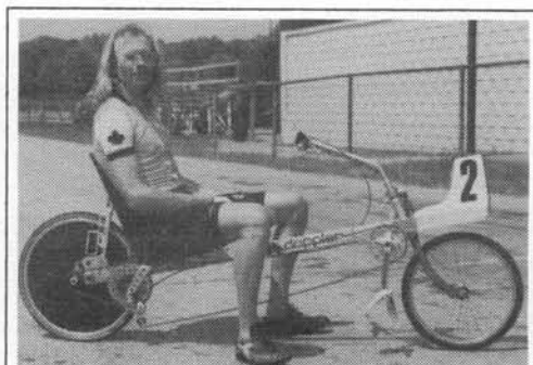
Figure 1: Peter Heisch on the 11-kg Doppler. Short handlebars require a lean-forward riding position. Main frame tube extends ahead of head tube to support fairing.
