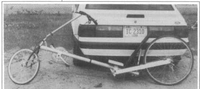
Figure 5 Bill Murphy's home-built recumbent. Head-tube angle, height, seat-back angle and bottom-bracket position are all adjustable. (Photo: Mike Eliasohn)
