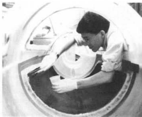
Figure 3. Lay-up of rear hatch
