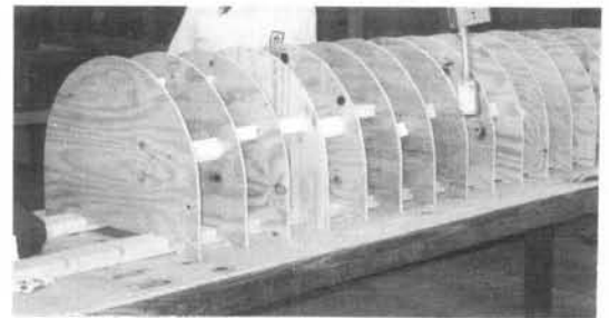
Figure 3. Initial Step in Male Plug Construction.
