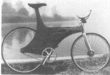
Original monocoque with first alloy monoblade
