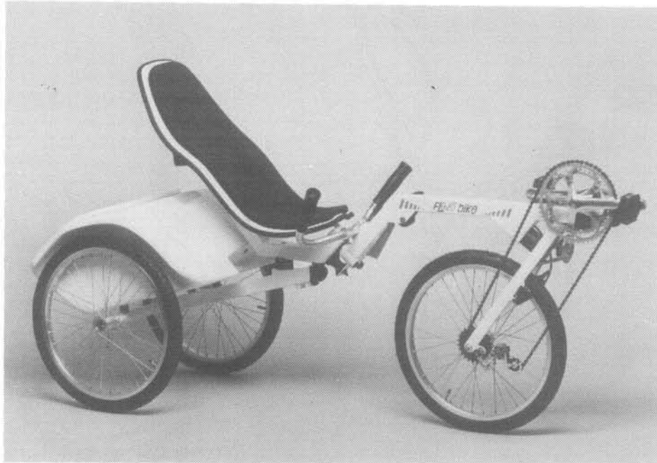
The Flevo conversion to a load-carrying tricycle.
