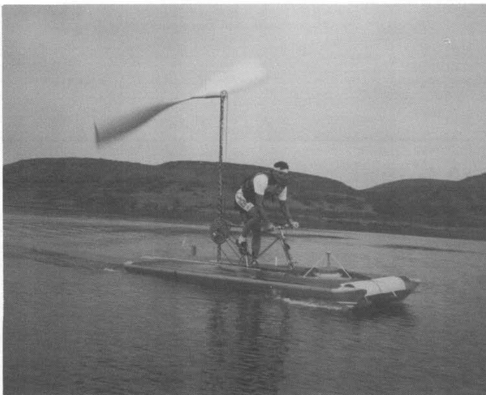
Richard Byrne has been the main engine for both Dragonfly II and III . At this point, the craft is just about to rise past "hump." Hump is the transition from being in the water to being on top of it.
