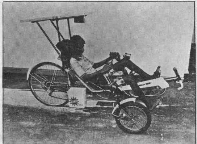
4 - The solar-photo-voltaic panel, batteries, and motor are a non-essential sophistication on this independently-three-wheel suspended recumbent trike for town running. It is convertible in about half an hour into an out-of-town commuter bike, still with independent wheel suspension.
