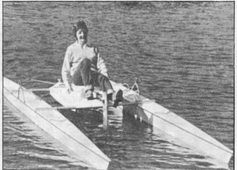
Hydra-Products' pedal-powered, propeller-driven Water Strider I.
