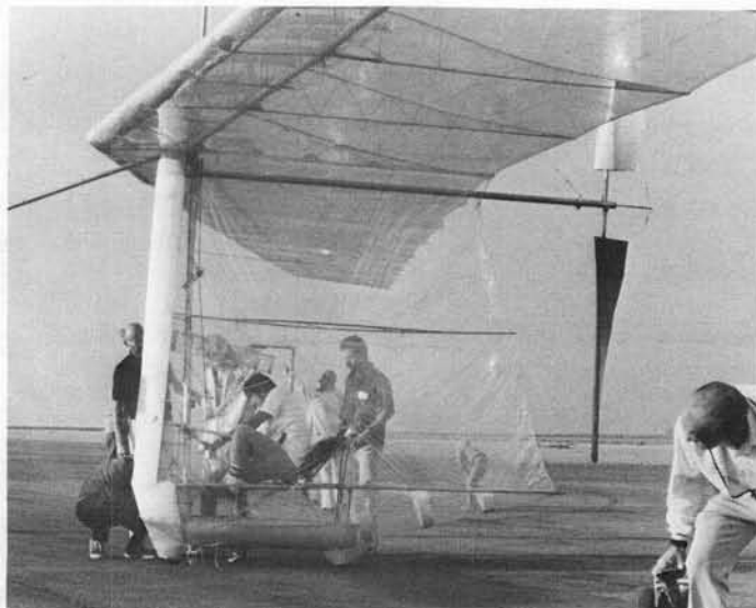
Side view of the fuselage shows the pedals mounted to the support pylon and the reclining seat.
